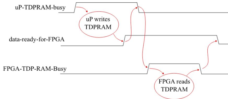
Asynchronous timing diagram of a flags-based protocol for safe data transmission through the TDPRAM of the CB
