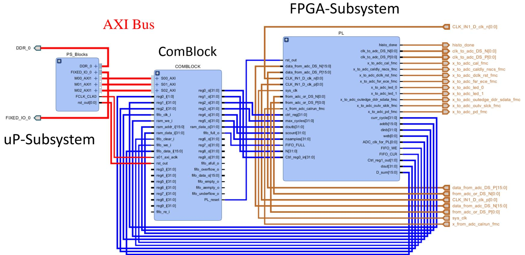
Custom connections with the FPGA-subsystem
